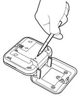
Using a ballpoint pen, briefly push and release the 'learn button' on the back of Alarm 2.The red LED next to the learn button will flash briefly then light up for approximately five seconds.
