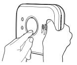
The red LED on Alarm 2 will flash to indicate that it has been 'learned-in' successfully. If the test button is not pressed quickly enough, the 'learn-in' process will fail. If this happens, repeat the process. To complete the installation fit Alarm 2 into position.
